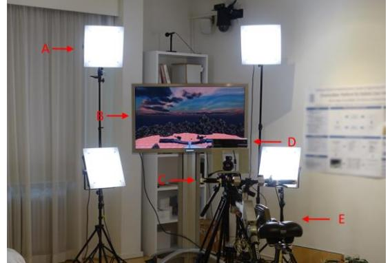
Figure 1: System Setup. A: Face Illumination, B: Display, C: Handlebar and Brake, D: Camera, E: Physical Exergame Controller
