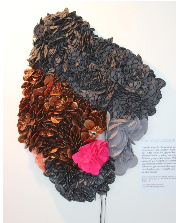
Fig. 1: Lomelia interface: A group of shells is connected to one of ten servo motors. To optimize detection of facial expressions, a frontal image is required, therefore a camera is mounted next to the pink flower acting as an eye catcher.
