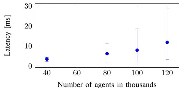
Fig. 3: Test with different numbers of agents, eight middleware nodes and seven runtime environment.
