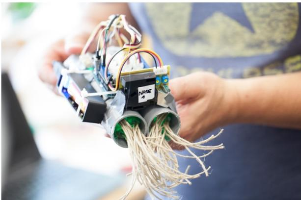
**Figure 4:** Prototype based on the whiskers of a mouse.
