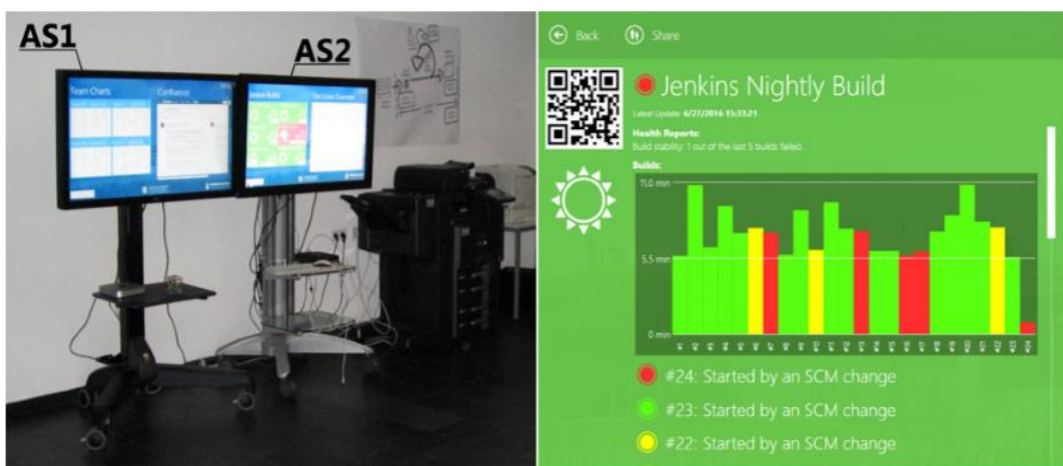
Figure 1. Left: The installation setup of both Ambient Surfaces in a common room on the ground floor; printers, whiteboards and the stairway to the upper level are in this area as well. Right: A custom visualization showing a build summary for a specific Jenkins job.
