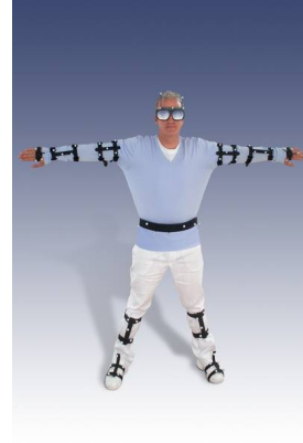
Abbildung 2.6: ART (2008) Motion Tracking Targets
