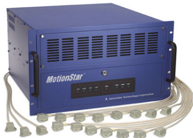
Abbildung 2.2: Ascension MotionStar Electromagnetic System
