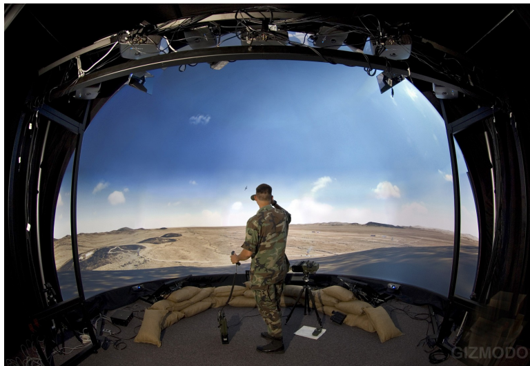
Abbildung 3.1: Ultra-high resolution multi-projector VR-System at Nellis Air Force Base in Nevada
