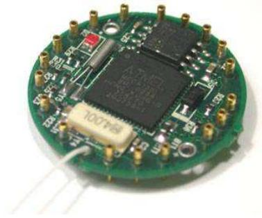
Abbildung 2: Berkeley Mote, MICA2Dot Implementation, Quelle: Crossbow Technology, Inc
