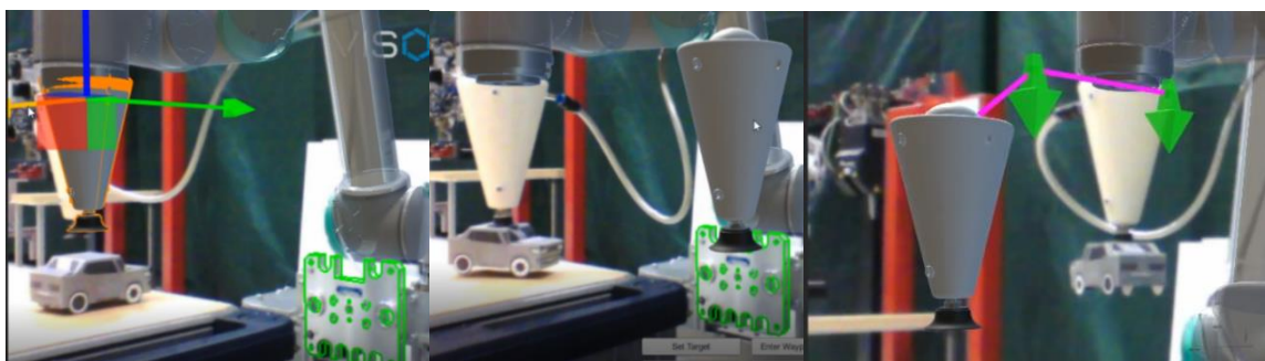
Figure 5-9 Execution of a pick and place task with the MR application
