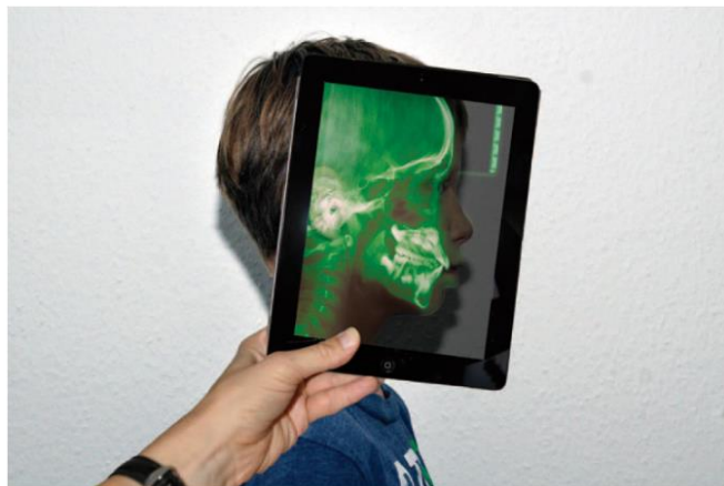
Figure 2-6 "Magic lens" type MR effect done with handheld device [4]
