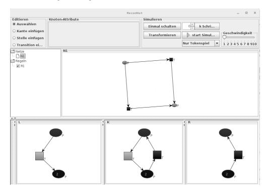
Figure 7: ReConNet: Graphical editor for reconfigurable Petri nets
