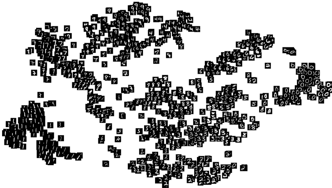
Figure 2.2: A latent space for the MNIST Dataset which shows how similar pictures achieve similar representations in a two-dimensional latent space [7]
