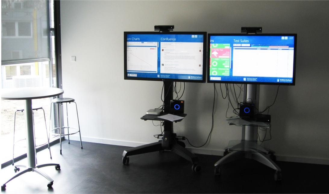
Figure 2.: Both Ambient Surfaces at their installation location, equipped with two Microsoft Kinect v2 sensors.
