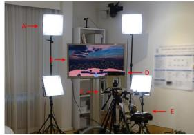
Figure 1: System Setup. A: Face Illumination, B: Display, C: Handlebar and Brake, D: Camera, E: Physical Exergame Controller
