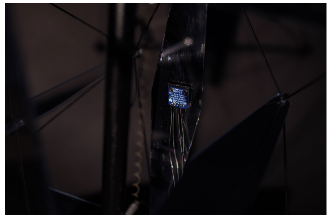
Figure 9: The SGP30 sensor is attached on the backside of the tensegrity strut.
