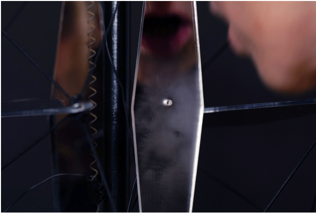
Figure 4: The user’s exhalation triggers the interactive mirror.
