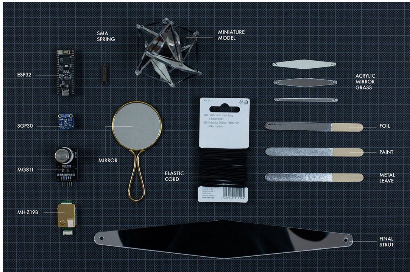
Figure 6: This picture illustrates materials, electronic components, and miniature model.
