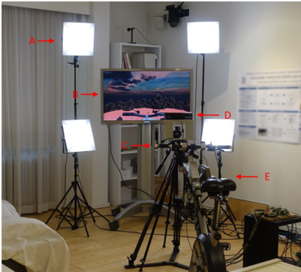
Figure 3.5: Physical setup for ES2: (A) illumination lamps; (B) frontal display; (C) rotatable handlebar, gear and brake; (D) Kinect Camera; (E) physical exergame controller (ergometer).
