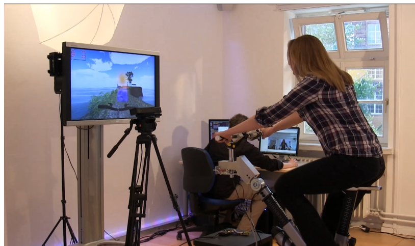
Figure 1.1: The EmotionBike, a cockpit-scenario as combination of an enhanced ergometer with a rotatable handlebar, a frontal camera and a video game.
