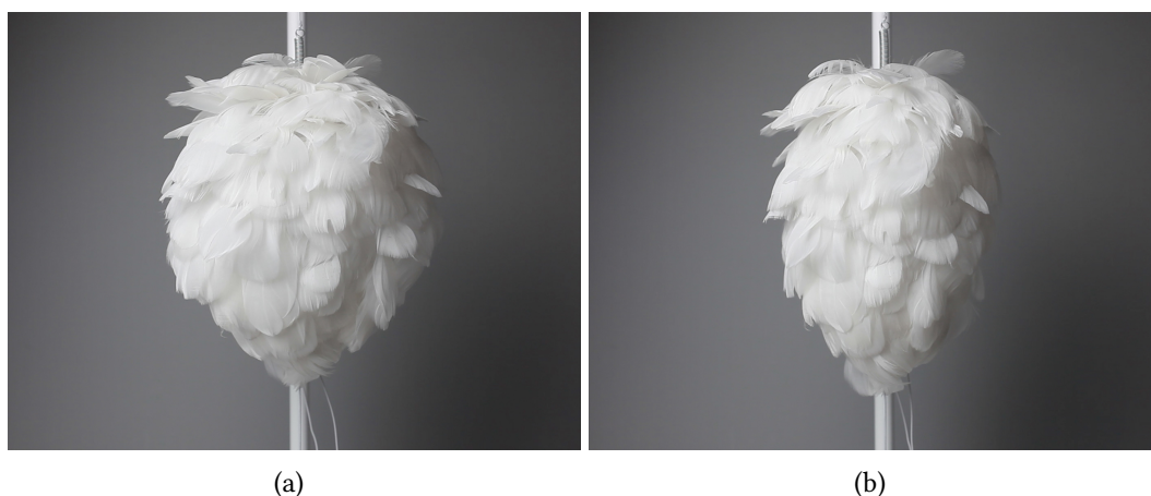
Figure 5.14 When PM-2.5 values are less than 35 \mu\text{g}/\text{m}^3 , the species-mimicking interfaces simulates a breathing and singing behaviour: (a) the state of inhalation, when the SMA spring is heated, (b) the state of exhalation, when the SMA spring is cold.
