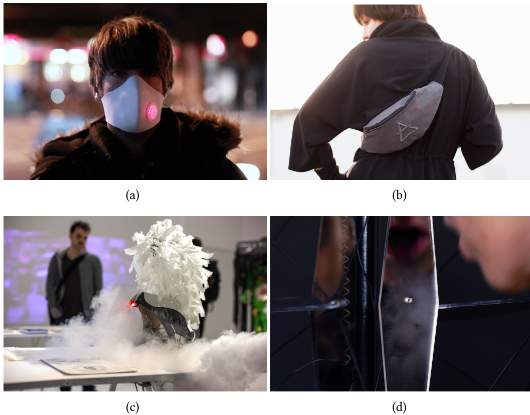
Figure 4.6 Preliminary studies conducted by the author to illustrate different types of interactions with the state of the air. Top: interactions through the use of (a) an illuminated mask that demonstrates the air quality of the near surroundings to other individuals in a public space and (b) a bag with a thermochromic symbol for air visualising two levels of air quality. Bottom: interactions involving manipulation of the atmospheric condition through the use of (c) vapour from an e-cigarette to impact the state of the air through particle concentrations and (d) exhalation to affect CO 2 concentrations.
