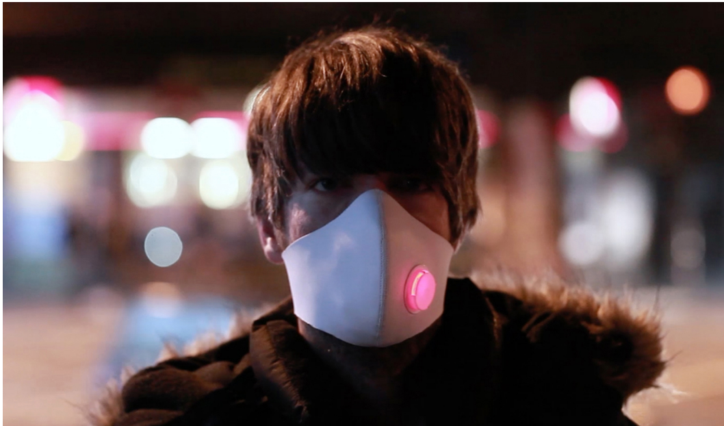
Figure 2.3 The Air Mask , a speculative design to monitor urban air pollution and to inform other citizens about the state of the air (Broscheit, 2020). The author developed the mask as part of a collaborative project at the Hamburg University of Applied Sciences in 2015.
