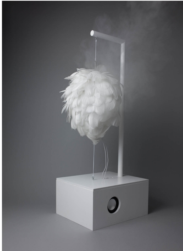
Figure 5.13 The initial sentinel species-mimicking interface, entitled Ivory , by Broscheit et al. (2019). The interface measures particles in the near surroundings and aims to convey the detected information through the use of a feathered, shape-changing surface enriched with sound. The interface dimensions are 600 mm height x 200 mm width x 240 mm depth.
