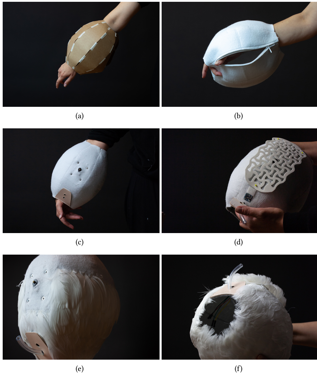
Figure 6.6 Impressions from the prototyping process of the sentinel species-mimicking interface: (a) the paper prototype, (b) fabric case with zipper, (c) integration of sensors and servo motor, (d) placement of the auxetic structure, (e) feathering process, and (f) the final interface.
