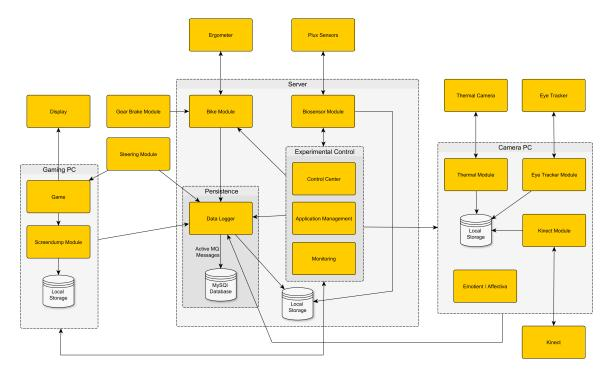
Figure 3.7.: Logical Deployment Diagram of the System Components
