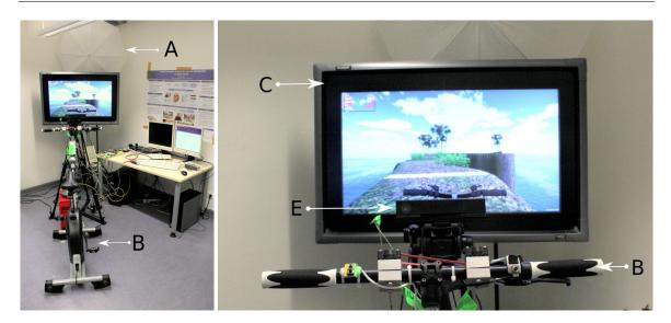
Figure 3.4.: Hardware Setup of the EmotionBike (Müller et al. 2015): Face Illumination Lamp (A), Cycling Game Controller (B), Screen (C) and Camera (D)
