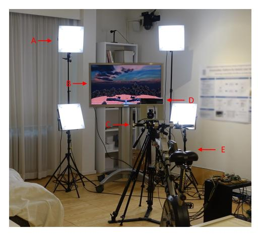
Figure 3.10.: System Setup. A: Face Illumination Lamps, B: Display, C: Rotatable Handlebar, Gearshift and Brake, D: Kinect Camera, E: Physical Exergame Controller (Müller et al. (2017a), <sup>©</sup>2017 IEEE)
