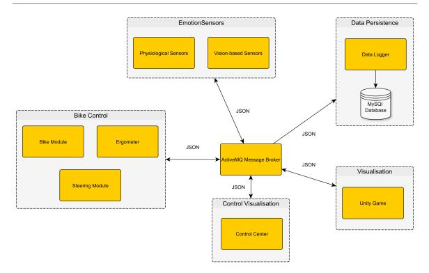
Figure 3.6.: Loosely Coupled System Design using a Blackboard Architecture
