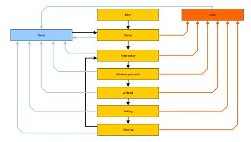
Figure 3.8.: Status of Nodes (Black: normal transition, Blue: reset triggered by the external monitoring component, Red: internal error)
