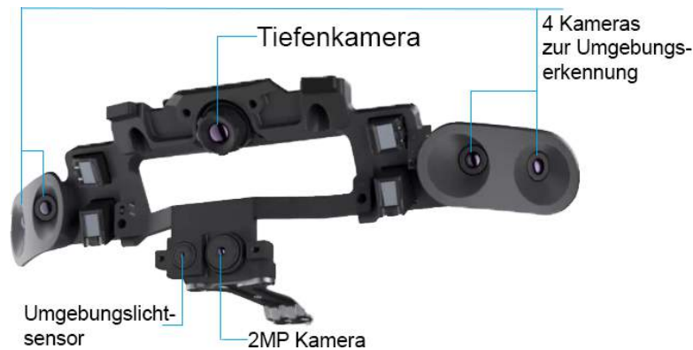
Abbildung 2.10: Sensoren Quelle: https://developer.microsoft.com/en-us/windows/mixed-reality/hololens_hardware_details (07.01.2018)
