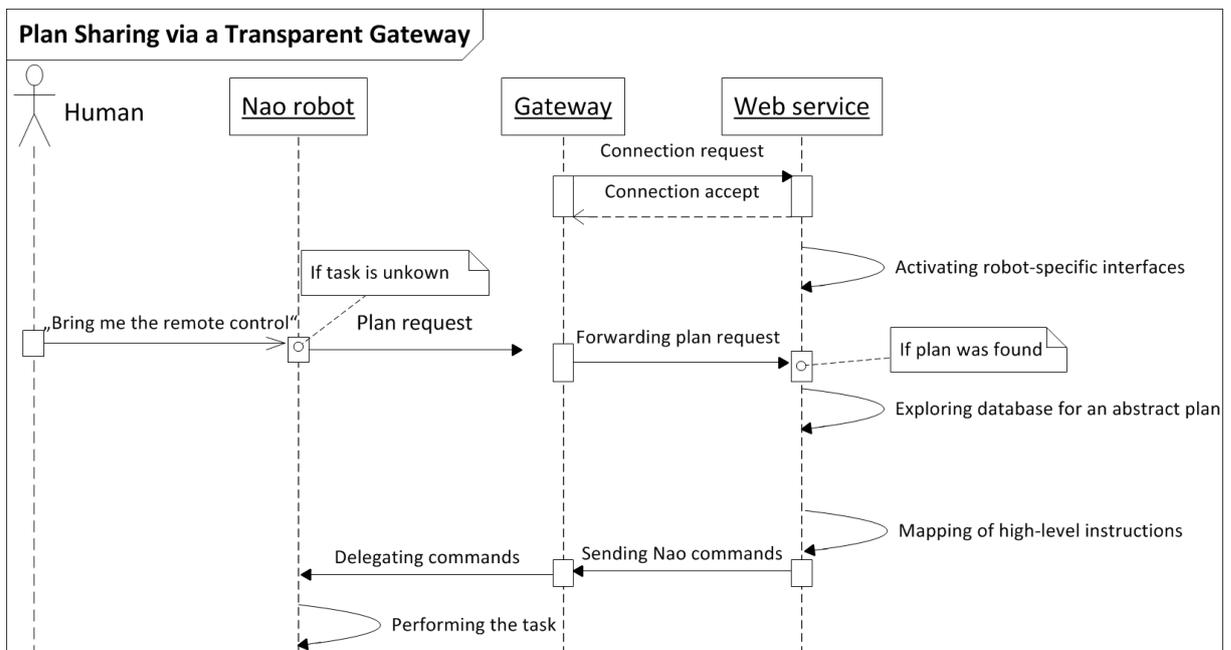
Figure 4.8: Sequence diagram for the transparent gateway approach
