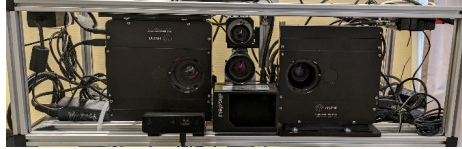
Fig. 1: MSI image acquisition setup. Filter wheels with bandpass filters are attached to the SWIR (left) and near infrared (NIR) (right) camera. The UV sensor is placed in the top center, the RGB sensor underneath.
