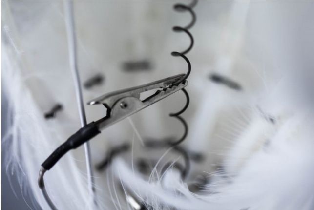
Figure 2: The shape memory alloy spring is placed in the center of the construction to generate the kinesis of the prototype.
