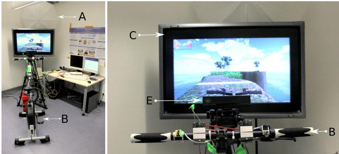
Figure 3.4.: Hardware Setup of the EmotionBike (Müller et al. 2015): Face Illumination Lamp (A), Cycling Game Controller (B), Screen (C) and Camera (D)
