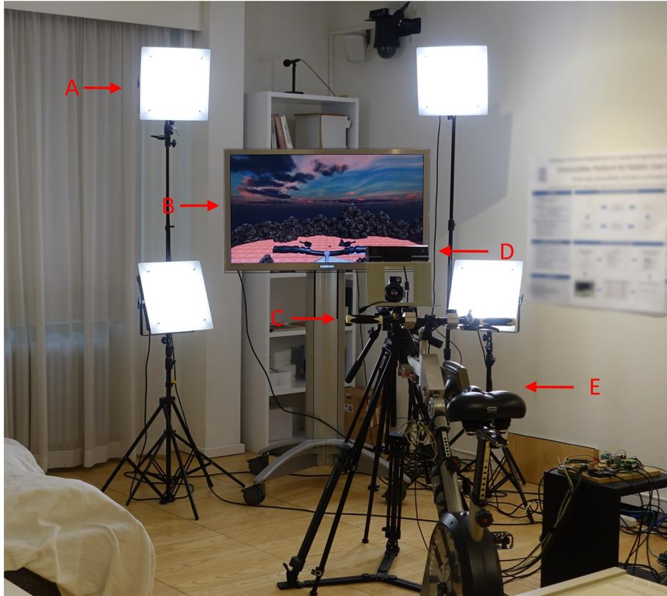
Figure 3.10.: System Setup. A: Face Illumination Lamps, B: Display, C: Rotatable Handlebar, Gearshift and Brake, D: Kinect Camera, E: Physical Exergame Controller (Müller et al. (2017a), ©2017 IEEE)
