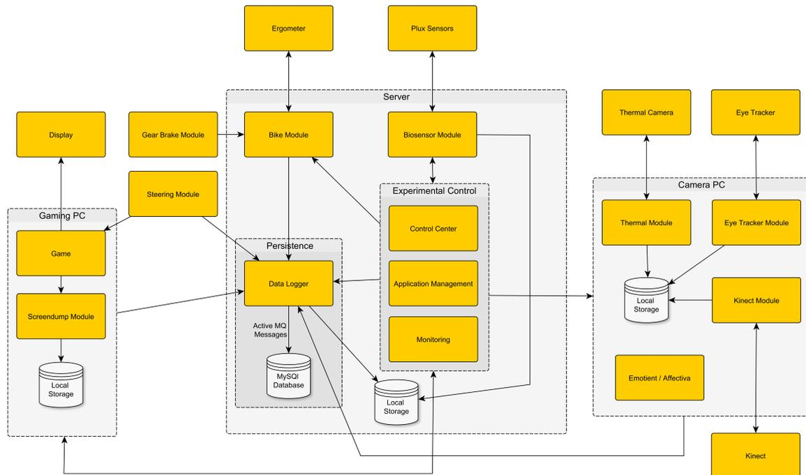
Figure 3.7.: Logical Deployment Diagram of the System Components
