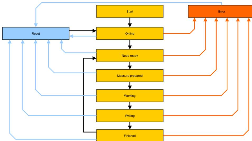
Figure 3.8.: Status of Nodes (Black: normal transition, Blue: reset triggered by the external monitoring component, Red: internal error)
