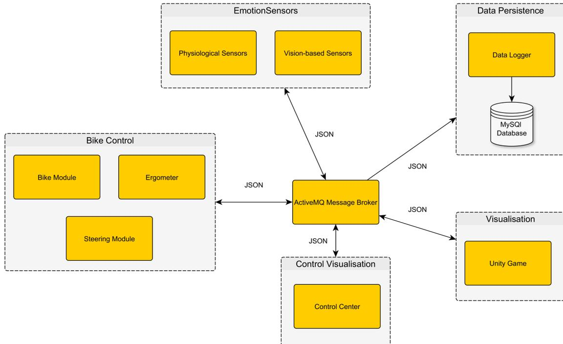
Figure 3.6.: Loosely Coupled System Design using a Blackboard Architecture
