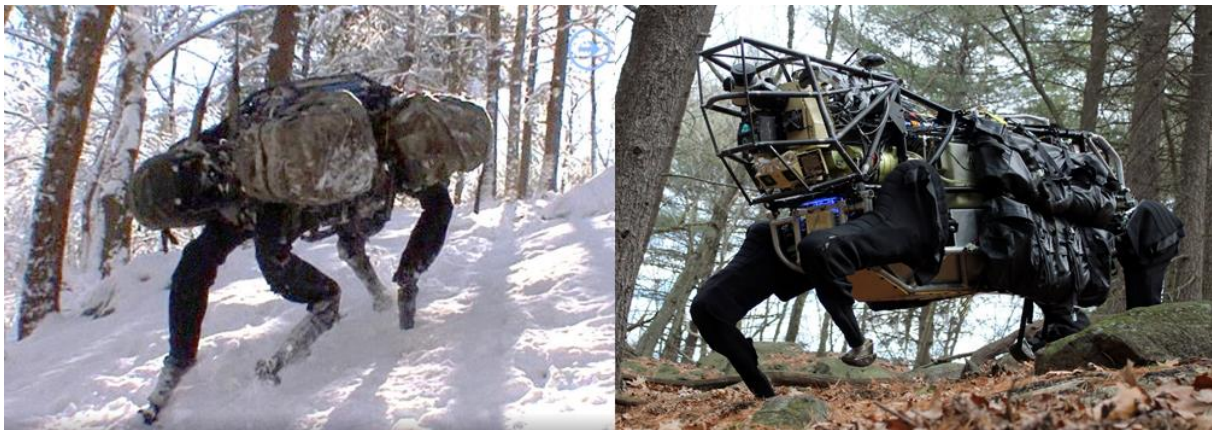
Abbildung 2-1 Boston Dynamics BigDog (links), AlphaDog-LS3 (rechts) [Bos10] [Bos13]
